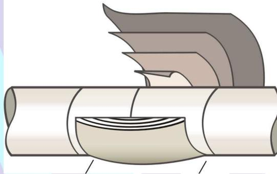
$$L_{(\text{min.})} = 16 \cdot E_{(\text{Espessura de Parede do Tubo})}$$
